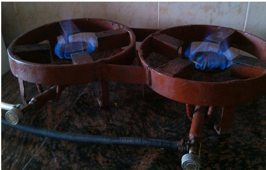
Fig. 1.5. Biogas flame from a table top double burner.
